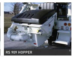
Putzmeister's robust, yet lightweight EZ Clean Out RS 909 hopper is engineered for performance and durability. Offering 19.4 ft<sup>3</sup> (550L) capacity, the hopper uses one remixer paddle motor and grate-mounted vibrator. An innovative RFID safety switch incorporated in the hopper disables the machine when the grate is opened.
