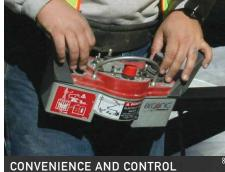
The Automatic Frequency Management (AFM) system on the standard HBC proportional radio remote ensures minimal interference with other frequency transmitters. A fully proportional cable remote is also standard. Unlike other remote control systems, the radio and cable remote systems are independent, offering redundancies to ensure proportional operation with either the radio or cable remote.
