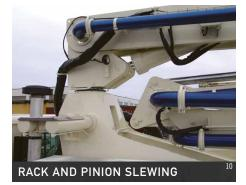
The 38Z-Meter boom features a simple mechanical rack and pinion design for improved weight distribution and easy serviceability. Specially designed teeth in the system offer smooth rotation and prevent backlash in the swing gears.
