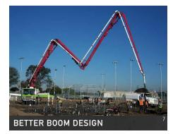
Robust and more resilient, Putzmeister's "smart design" boom incorporates welding seams below the edge of maximum stress. The boom is engineered to offer the flexibility to adapt to different loads and features more straight pipe for a less stressful concrete flow and longer wear on parts. The Multi-Z configuration handles space restrictive areas and can pump even if the boom is not fully extended.
